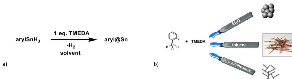
**Figure 1.** a) Synthesis of aryl decorated nano particles **aryl@Sn** *via* dehydrogenative coupling reaction of aryltin trihydrides. b) Morphology fine tuning of *o*-tolyl@Sn.
