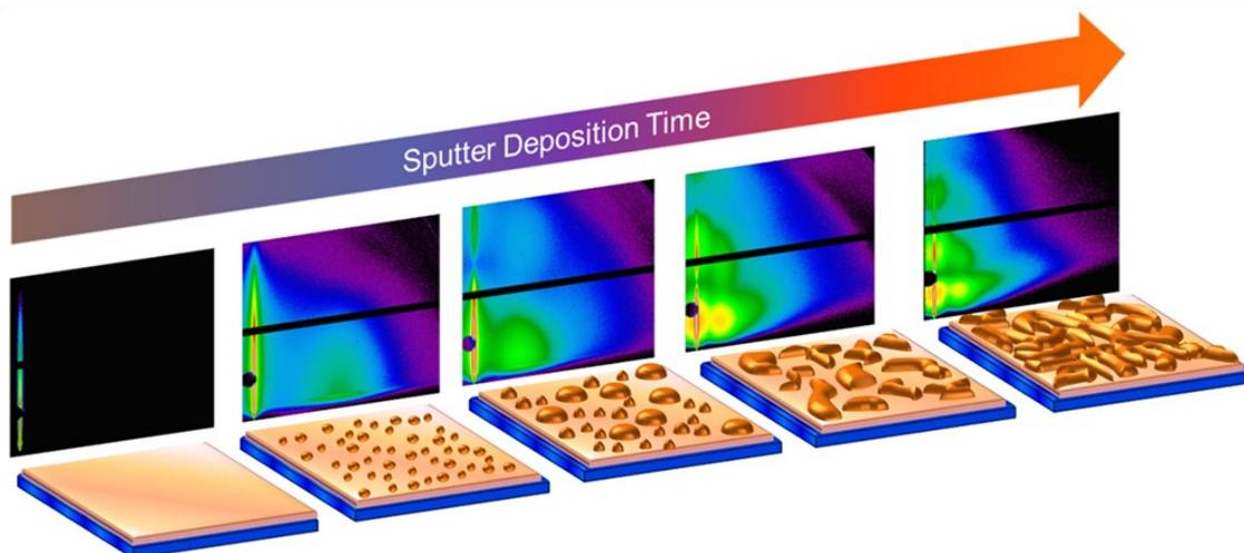
**Fig. 1:** Nucleation, condensation and growth of a gold layer on top of an organic substrate is observed in real-time during sputter deposition using in-situ  $\mu$ GISAXS [3].
