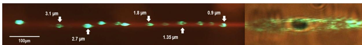
Figure 2 Left: Sizing and filtering of multilamellar phospholipid (DPPC) vesicles; system-parameter result in corresponding filter pore size of 0.9  $\mu\text{m}$ . Right: Cell deformation in trap-mode. Deformation force = 5.2 pN
