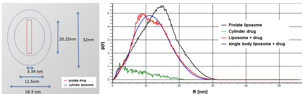
**Figure 1:** Study of a liposome drug carrier system. Data, obtained from a SAXS-measurement, yielded with aid of single body simulation (simulated Pair Distance Distribution Function on the right side) in the depicted model of the drug-loaded liposome (on the left side).
