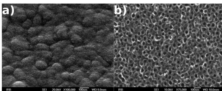
**Figure 1:** SEM image of Ti substrate (a) and TiO<sub>2</sub> nanotubes array (b) obtained by anodization.
