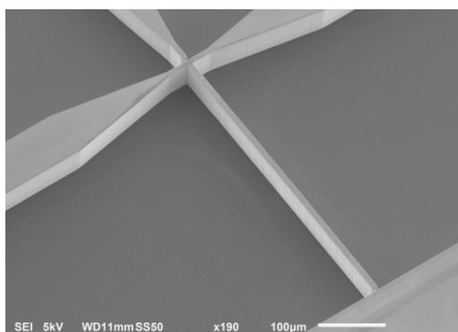
Fig.1 – SEM picture of the produced Si mould
