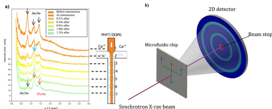
**Figure 1:** Time resolved SAXS experiments displaying the dynamic structural transitions in the interiors of PHYT/DOPG nanoparticles, a) hydrodynamic focusing chip with green circles indicating the positions at which SAXS was measured b) the combination of microfluidic with SAXS.
