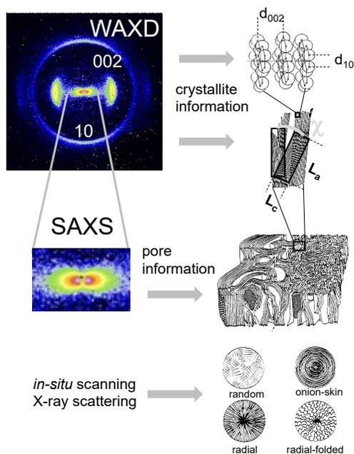
**Figure 1:** figureTypcial SAXS and WAXS image of a carbon fiber and the corresponding structure.
