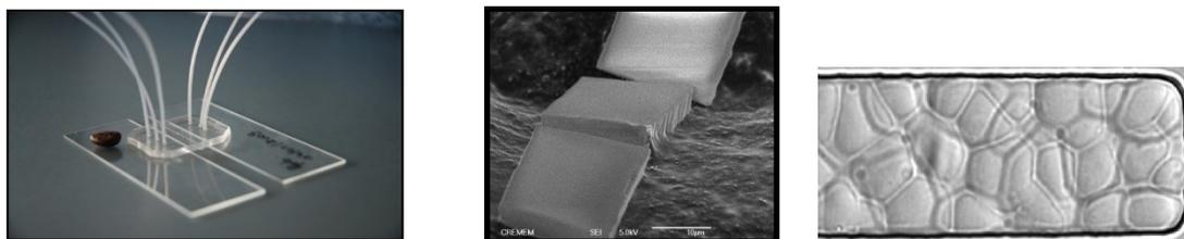
**Figure:** Left: microfluidic pervaporation for phase diagram screening. Middle: SEM view on a dense assembly of gold NPs. Right: nucleation and growth of colloidal crystals in a microfluidic pervaporation channel.
