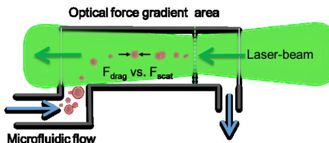
Fig. 1 Schematic presentation of the basic OFC principle
